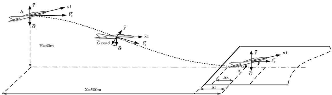
Figure 9 – UAV's state when landing
