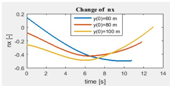
Figure 7 – Tangential overload
