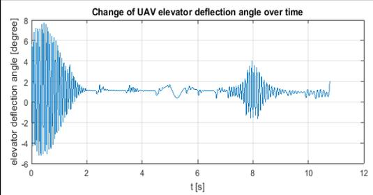
*Figure 17 – Change of UAV elevator deflection angle over time*
