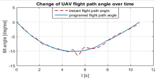
*Figure 16 – Change of UAV flight path angle over time*
