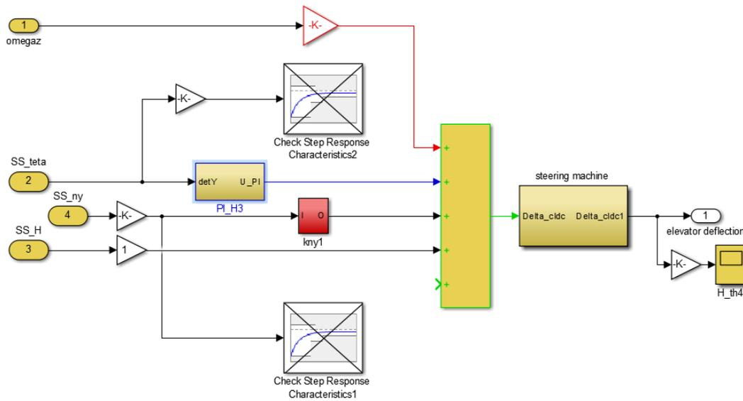
Figure 11 – The UAV 's pitch angle controller
