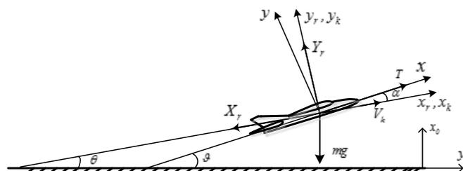
Figure 1 – UAV motion in vertical plane
