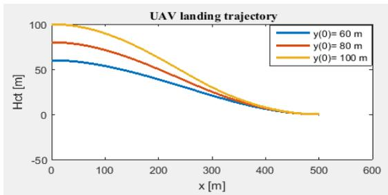
Figure 3 – Landing trajectory of UAV
