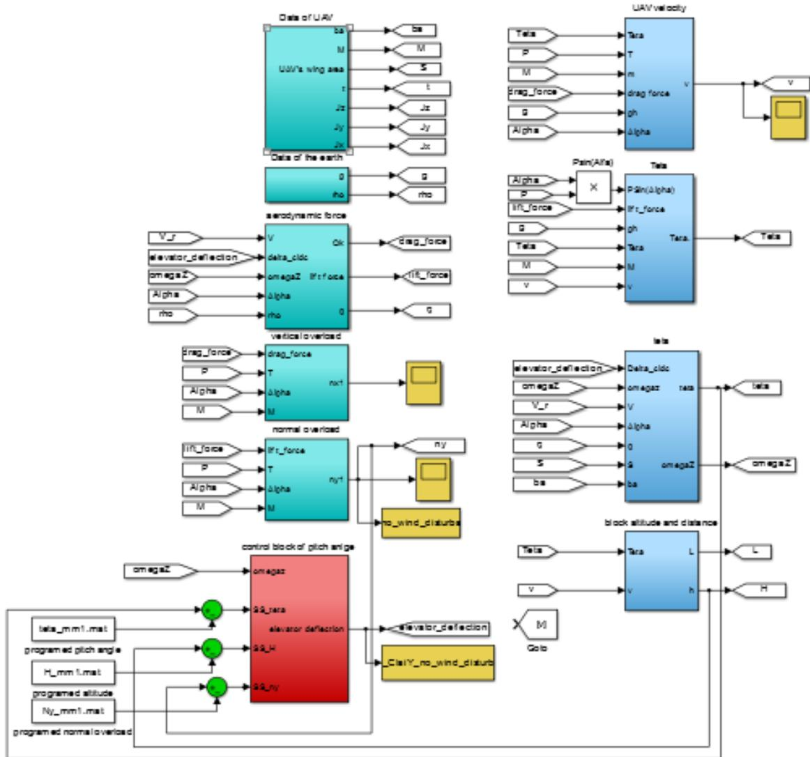
Figure 10 – Block diagram of closed loop of the UAV vertical motion
