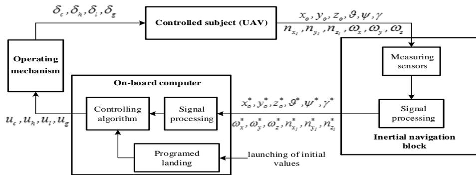
Figure 2 – Block diagram of closed-loop UAV landing controller
