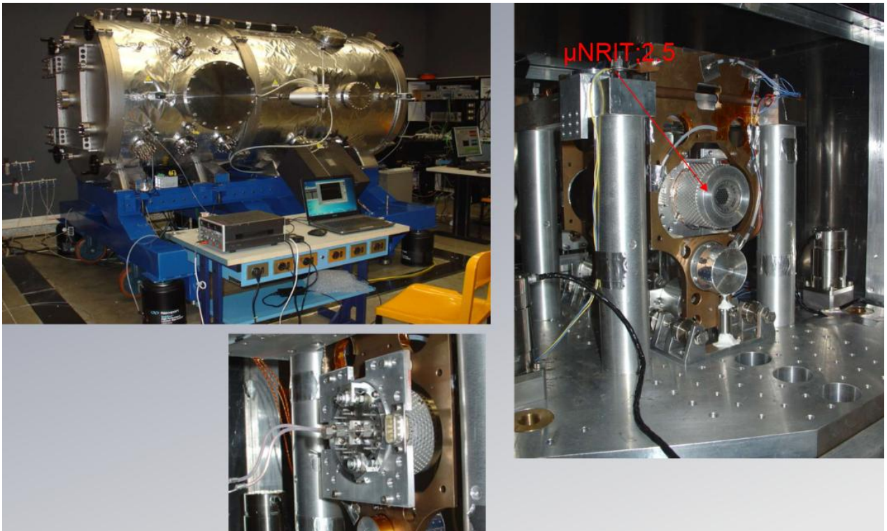
Figure 6 – High vacuum test stand (left) and two photos of the \mu N RIT-2.5 engine on the nano-balance facility of Thales Alenia Space for direct thrust measurements
